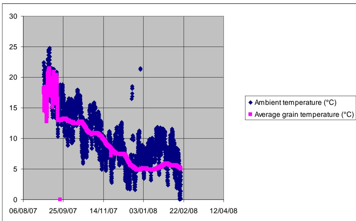
**Figure 28.** Temperature change in Bin 4 over time
