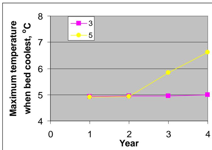
**Figure 16.** Odiham, cooling a 6 m bed to a target of warmest layer less than 5 °C with a diffstat at 3°C and 5°C. The maximum bed temperatures at end of cooling for each of the 4 years were sorted to show the pattern.
