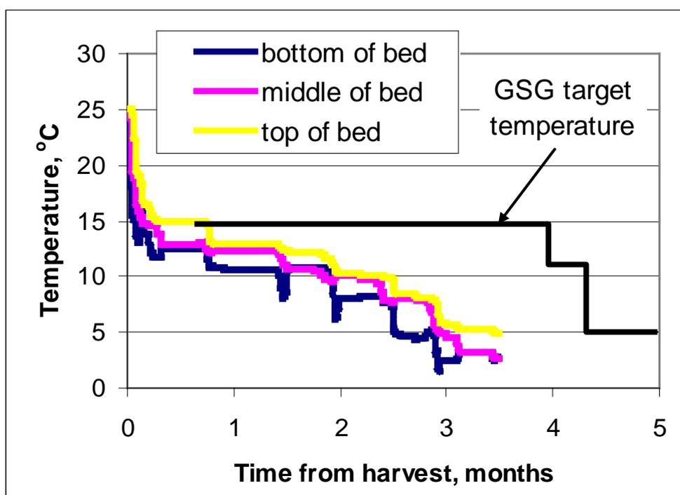
**Figure 17.** Time course of temperature at bottom, middle and top of a 4 m deep bed at Odiham in 1998, simulated with a differential thermostat set at 4°C comparing ambient temperature and average bed temperature.
