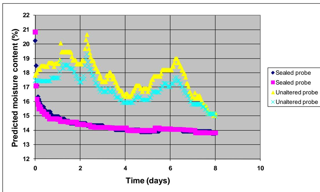
**Figure 32.** Predicted moisture content from unmodified probes and probes with the final modification
