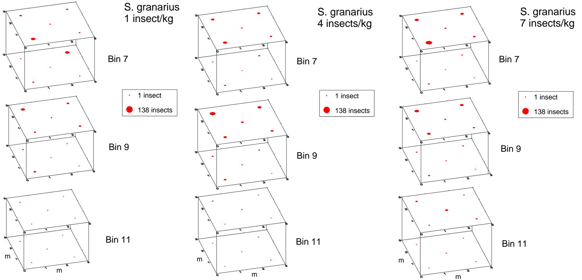
Figure 27. Distribution of insect trap catches across bin areas at the surface, 10 cm and 50 cm
