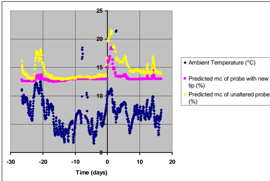
**Figure 30.** Predicted moisture content from modified and unmodified probes.
