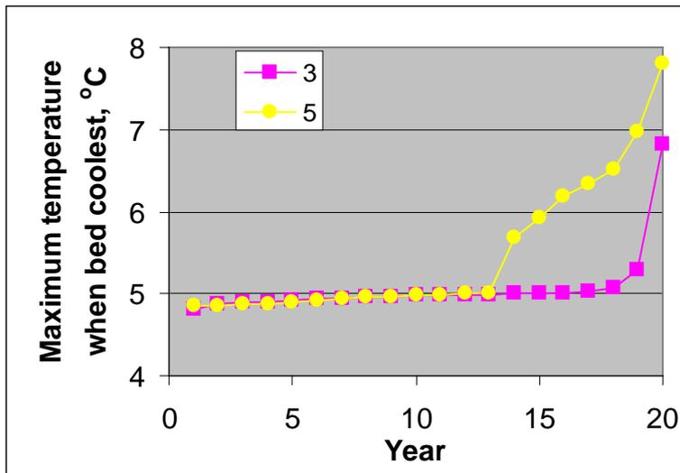
**Figure 15.** Waddington, cooling a 6m bed to a target of warmest layer less than 5 °C with a diffstat at 3 and 5 °C. The maximum bed temperatures at end of cooling for each of the 20 years were sorted to show the pattern.
